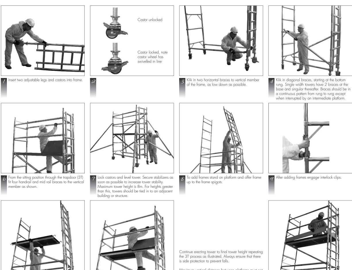
Fit trapdoor platform on appropriate rung. See tower illustration for guide.
