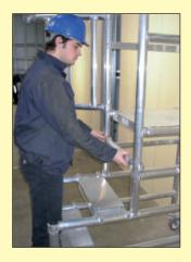
To work at the highest level fit platform on top rung and serrated climbing rung as shown.
