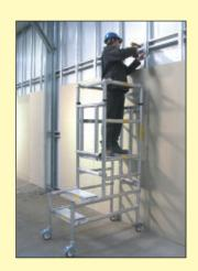
With the platform on the fourth rung the platform height is 1.17m, giving a reach height of 3.2m.
