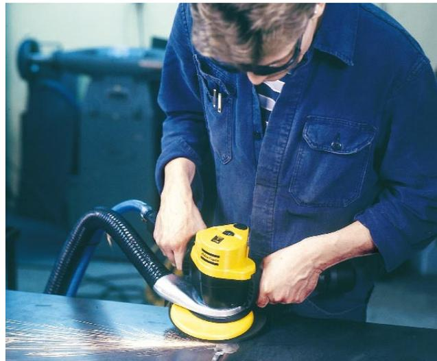
180 mm kit (7") fitted to heavy metal grinder. Turning the snap-in hood compensates for a decreasing grinding disc diameter.
