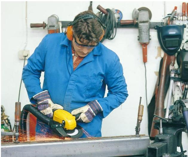
Tool in operation. Fine particles are efficiently captured. No "smell of grinding" any more. Heavy particles, not hazardous to your health, are hard to capture.
