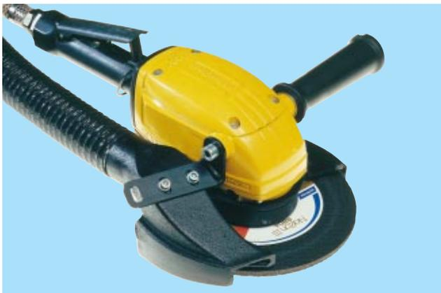
Extraction nozzle fitted to a modern heavy metal grinder.
