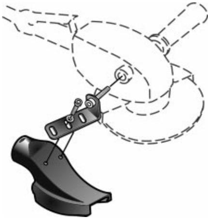
The adapter can hold the nozzle in two positions to match  $\text{Ø}180\text{mm}$  (7") or  $\text{Ø}230\text{ mm}$  (9") grinding wheels.
