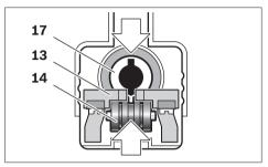
**Note:** If the grooves of the saw blade holder are not in the position shown in the figure or when the Precision-Control guide cheeks **13** are closed, then the saw blade **15** cannot be inserted into the stroke rod **17**. Briefly press the SDS clamping lever **19** toward the side and release it again.
